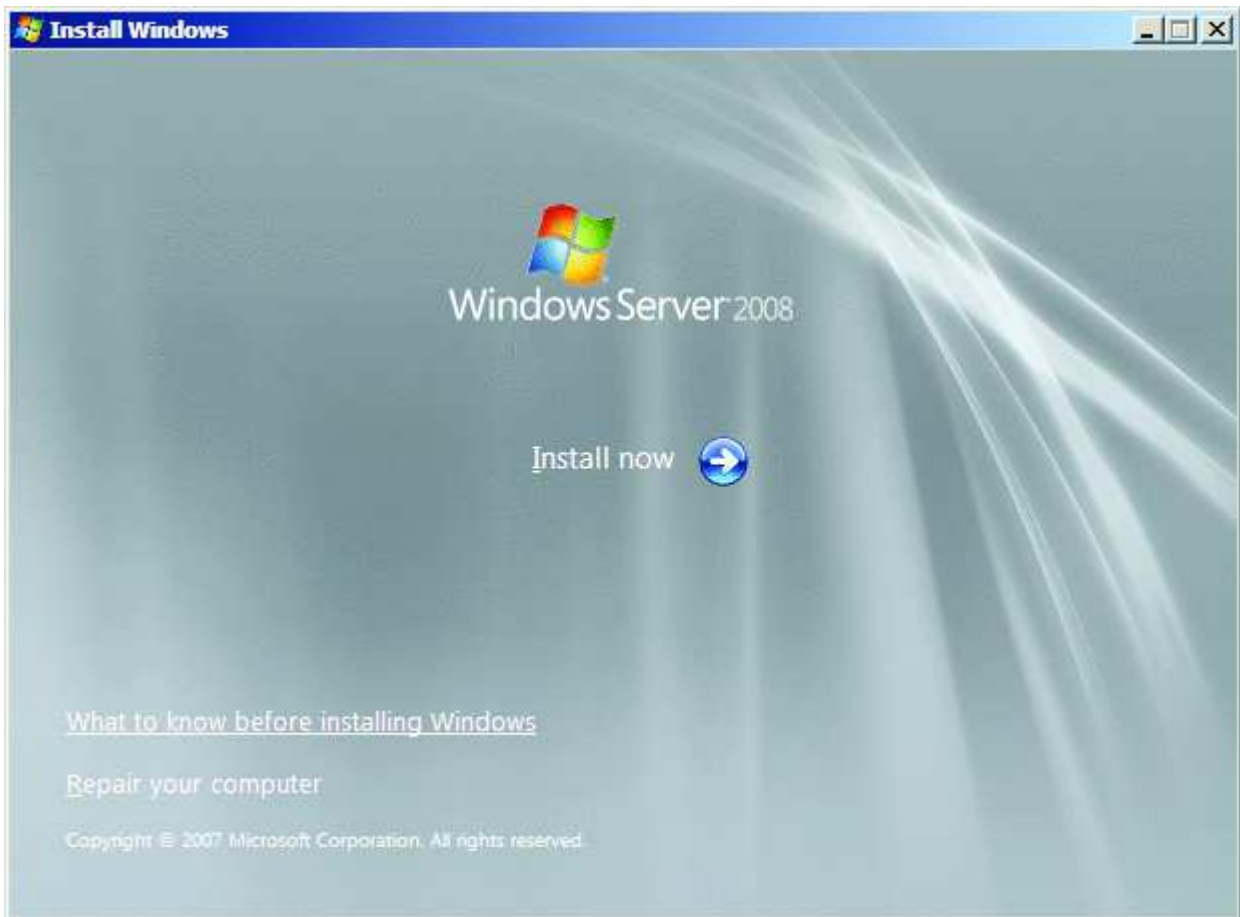
Figure 7 The Repair your computer option is available on the installation screen
