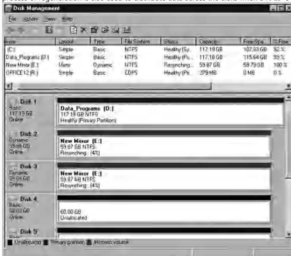
Figure 19-20 A newly created mirrored disk in the process of regeneration
